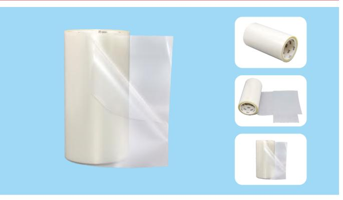
Acid resistance film is made of high performance PET film as the base material, coated with special acid and alkali resistant acrylic pressure sensitive adhesive. It has the characteristics of acid and alkali resistance, super corrosion resistance, high temperature resistance, no residual glue
