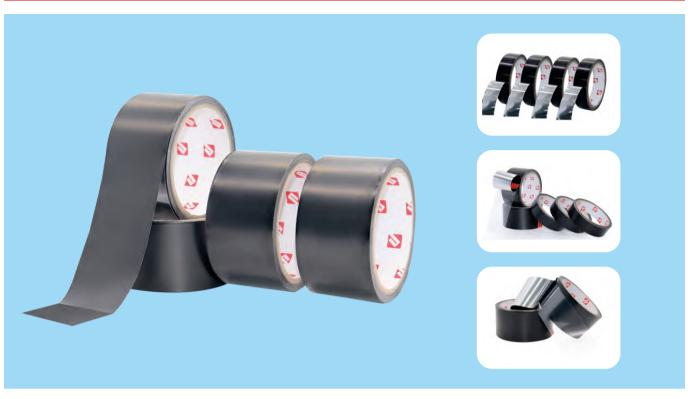
Nano carbon aluminum foil tape is based on high-performance aluminum foil for heat dissipation, The surface is compounded with nano-carbon, and then coated with acrylate functional heat dissipation adhesive.
